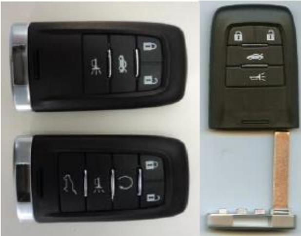
With the introduction of the 2010-11 9-5 and 2011 9-4X many new features were incorporated into the alarm system. The most noticeable is the Passive Entry Passive Start (PEPS) option.
