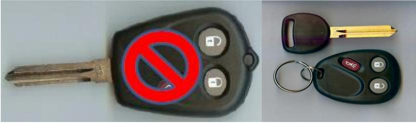
The 9-7X uses a PASS-Key III (PK3) alarm system, it uses transponder style key.
