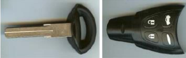
With the introduction of the 2003 9-3 Sport Sedan many new features were incorporated into the alarm system. The most noticeable difference was the new key/remote control that no longer utilizes a traditional key except for a door key that snaps into the key head. Depending upon the model and equipment levels it also became possible to open your windows or Convertible top remotely, activate halo lighting and activate a panic alarm.
